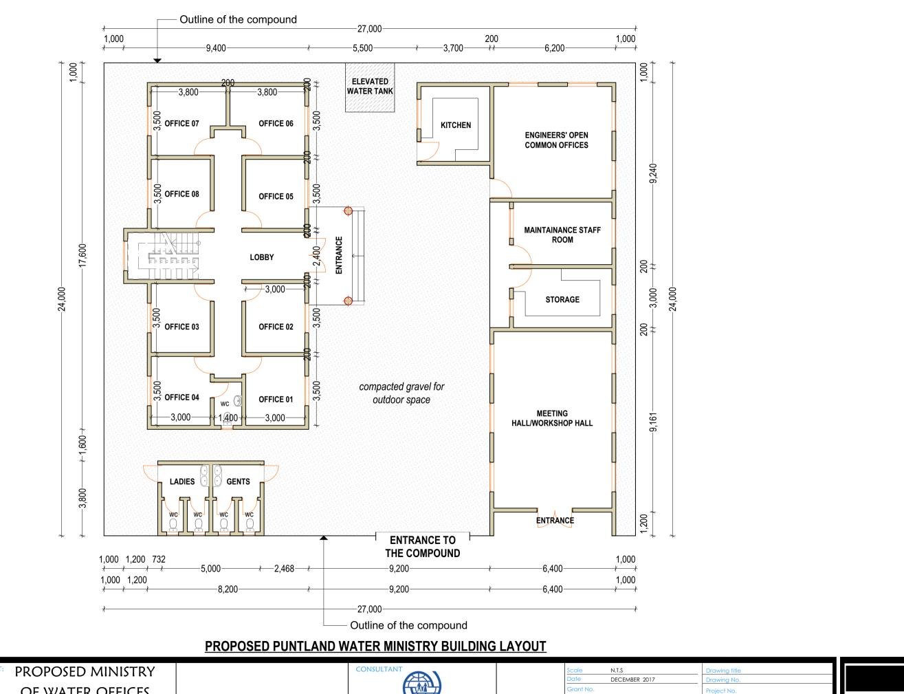
All dimensions are in mm unless stated Any discrepancies in the drawings should be eported to the consultants before the contractor commences work on site.
